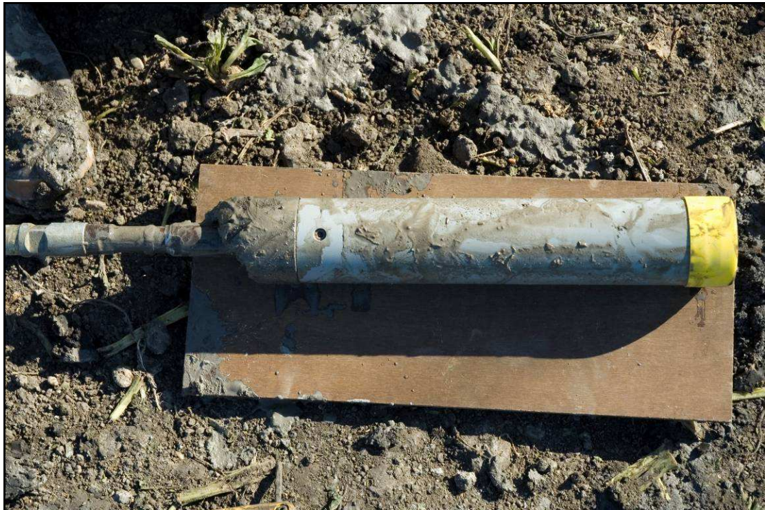
Fig. 1 The Van de Horst sampling equipment used for OSL sampling in channel sands
